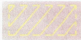
Very dangerous place at the railway crossing or at the junction
