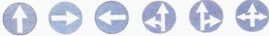
Ahead only Turn right Turn left Ahead or left Ahead or right Ahead or right or left
